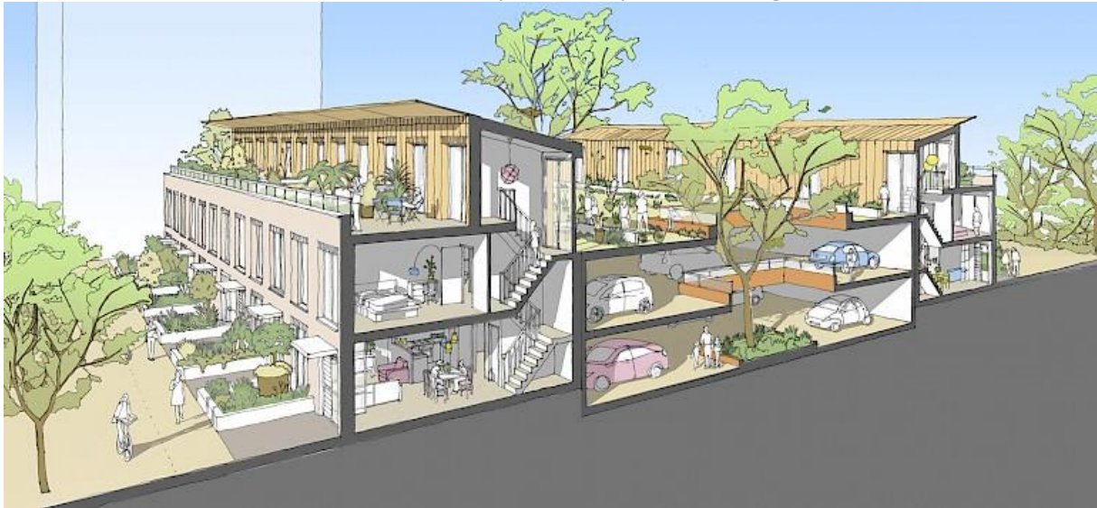
Double storey of Private Car parking located under raised private garden decks.
