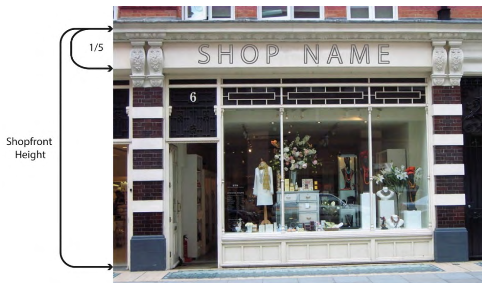
Figure 28: How to identify appropriate fascia board height.
