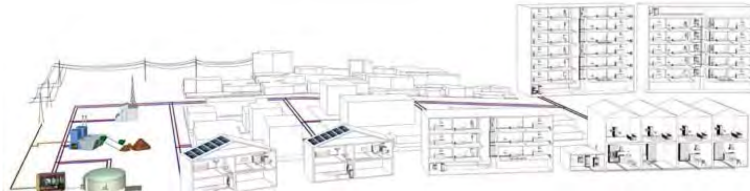
Figure 21: Schematic of a Typical District Heating Network
