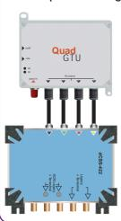
If you have a Quad GTU, the engineer will need to connect a DCSS switch to it, to allow you to receive Sky Q services.
